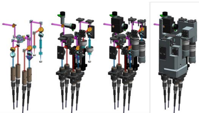
Fig 2: 800 & 1060nm free beam interferometer with fiber coupling, reference arm and two axis galvo-scanner
